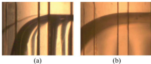
**Figure 8. Image of flooding in the gas chamber in FFMRs at different water flow rates: (a) FFMR I,  $d_G = 0.8$  mm,  $Q_L = 3$  ml/min; (b) FFMR III,  $d_G = 3.0$  mm,  $Q_L = 50$  ml/min.**
