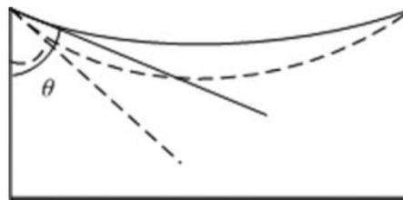
**Figure 16. Effect of channel wettability on the profile of falling film.**
