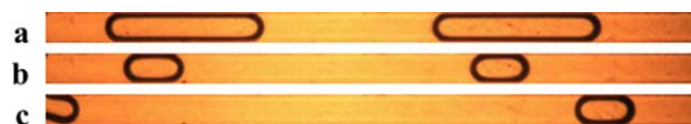
Figure 10. The relationship between the liquid slug length and liquid superficial velocity under 3.0 MPa, (a) j_G = 0.004 m/s, j_L = 0.0093 m/s; (b) j_G = 0.004 m/s, j_L = 0.0231 m/s; and (c) j_G = 0.004 m/s, j_L = 0.0463 m/s.
