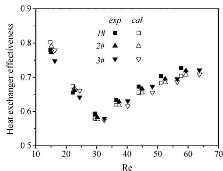
Figure 9. Calculated and measured heat exchanger effectiveness in the MCHES with two plates.
