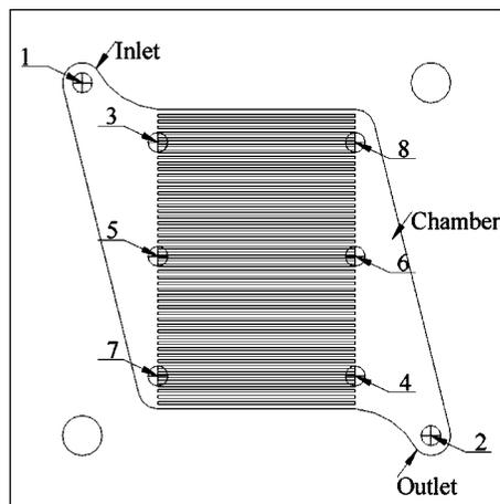
Figure 11. Schematic diagram of the microstructure for pressure measurement.
