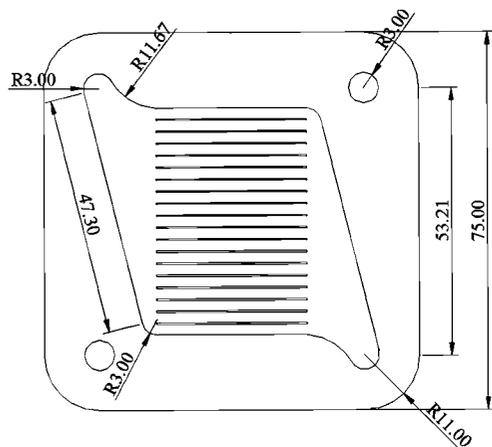
Figure 3. Geometry dimension of a plate of the MCHE.
