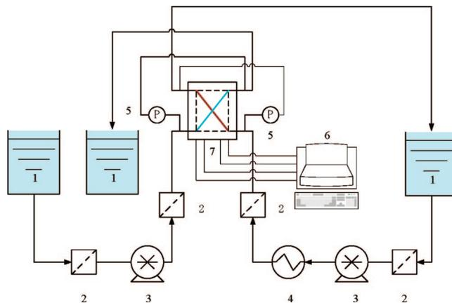
**Figure 1.** Experimental apparatus: (1) water tank; (2) filter; (3) water pump; (4) electric heater; (5) differential pressure transducer; (6) multiplexer and computer; (7) MCHE.
