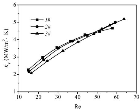
Figure 6. Volumetric heat transfer coefficient as a function of  $Re$  in microchannels.
