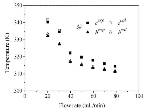
Figure 8. Calculated and measured outlet temperatures in the MCHES with two plates.
