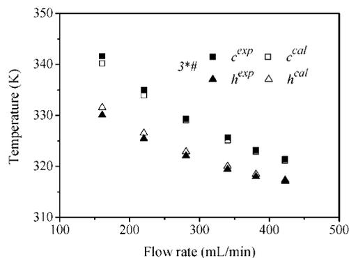
Figure 12. Calculated and measured outlet temperatures in the MCHEs with ten plates.
