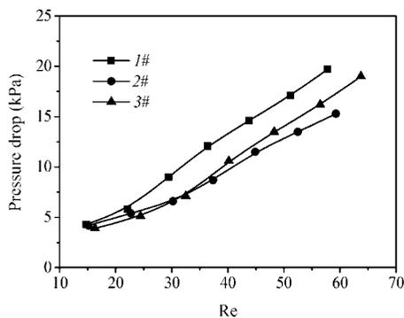
Figure 10. Measured pressure drop as a function of  $Re$  in microchannels.
