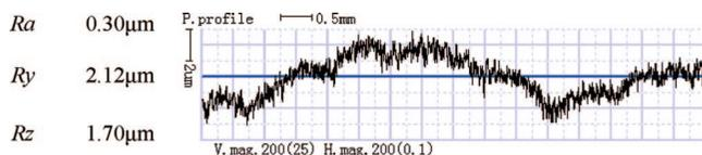
Figure 4. Surface roughness of etched area.
