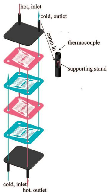
Figure 2. Exploded view of a counterflow MCHE with four plates.
