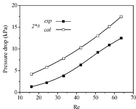
**Figure 13.** Calculated and measured pressure drop in one MCHE with ten plates.
