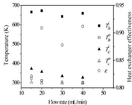
**Figure 14.** Outlet temperatures and heat exchanger effectiveness of MCHE 2.
